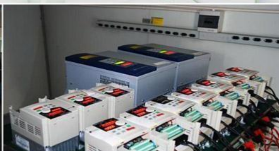
8. Protection functions & overload capacity testing.
