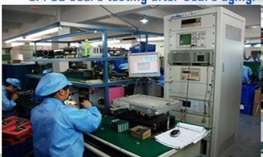
3. PCB board testing after board aging.
