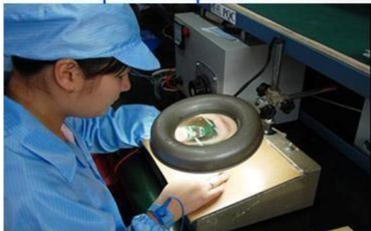
3. PCB board testing after board aging.
