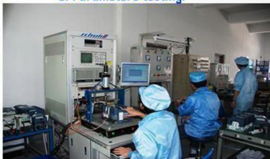
7. Final quality testing with load.
